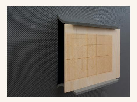
Laser on 3mm plywood clamped by shoe sole rubber nailed to a wall 13.5 x 18 cm (plywood)
